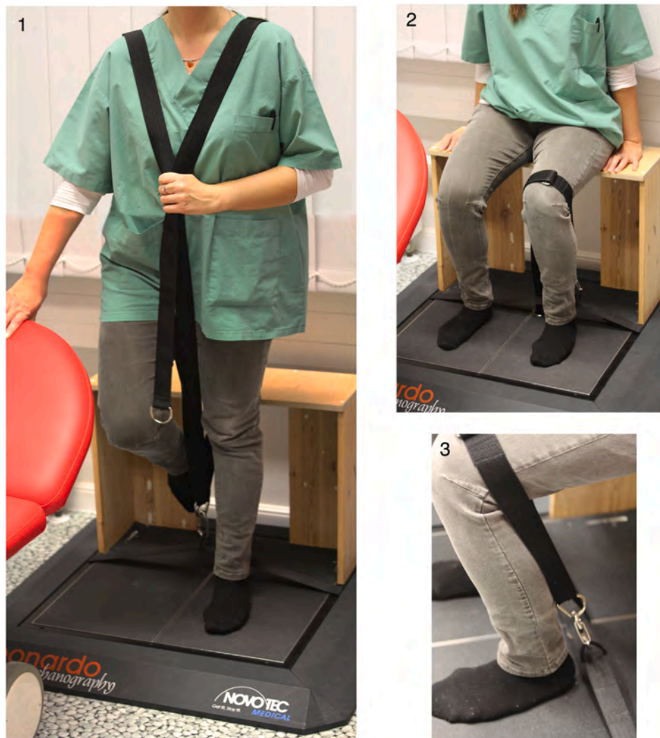
Fig. 2. Test setup: 1. measurement in knee extension 2. in knee flexion 3. fixation of the leg with a strap around the knee for measurement in knee flexion; ground reaction forces were determined over the two separate platforms for each leg.
